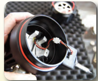
Carefully Separate Plug at the 3-Pin Connector
